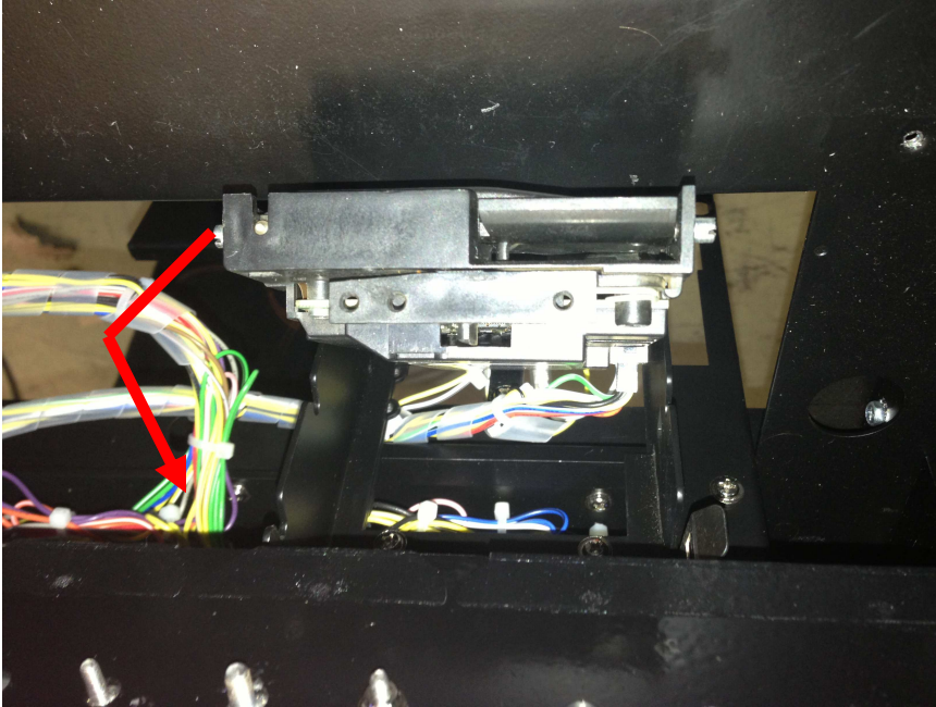
Figure 8: Removal of the coin acceptor
