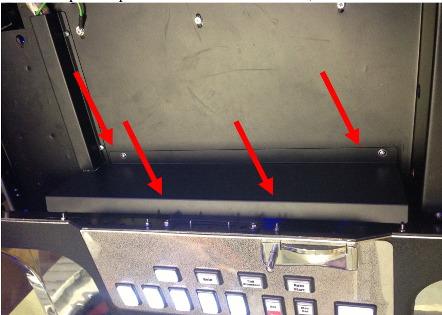
Figure 7: Coin Acceptor bracket position
