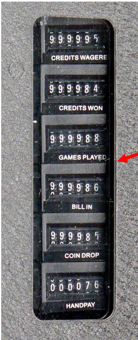
Figure 17: Hardware Meters Position in Machine
